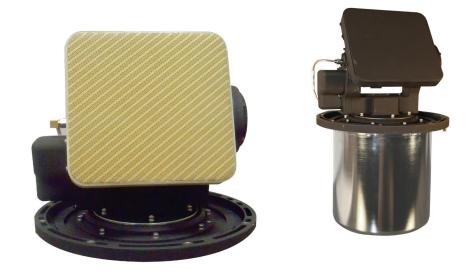
The AT-23 Directional Antenna is designed for use in airborne and ground Tactical Common Data Link (TCDL) applications. The AT-23 features a Dual Axis Positioner and a slotted waveguide array antenna. The slotted waveguide array has antenna gain of +23 dBi at the user output connector.
