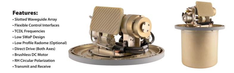
The AT-20 Dual Axis slotted waveguide array is designed for use in airborne and ground Tactical Common Data Link (TCDL) applications. The AT-20 features a Dual Axis Positioner and a slotted waveguide array antenna. The slotted waveguide array has antenna gain of 17 dBi at the user output connector.
